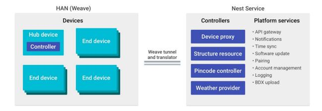
Devices in the HAN on the left provide non-real-time services and communicate with Nest Service on the right through the Weave tunnel and translator. The Nest Service on the right provides real-time services using controllers and platform services to manage devices in the HAN.
