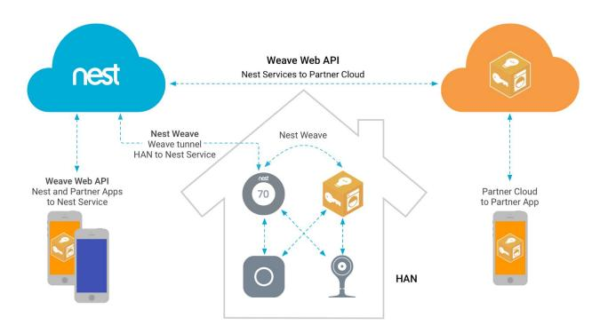
The Weave system works as a heterogeneous distributed computing system implemented on multiple types of hosts, such as battery-powered microcontroller-based devices, line-powered Linux-class devices, and powerful cloud-hosted services. The protocols interoperating between these hosts support a number of important capabilities including:
