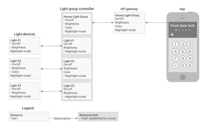
In this example, a light group controller manages a set of three lights in the HAN. The on/off, brightness, and (on some lights) color traits are managed by the controller passing update commands. The Nightlight mode setting for each light is published by the controller, and the
