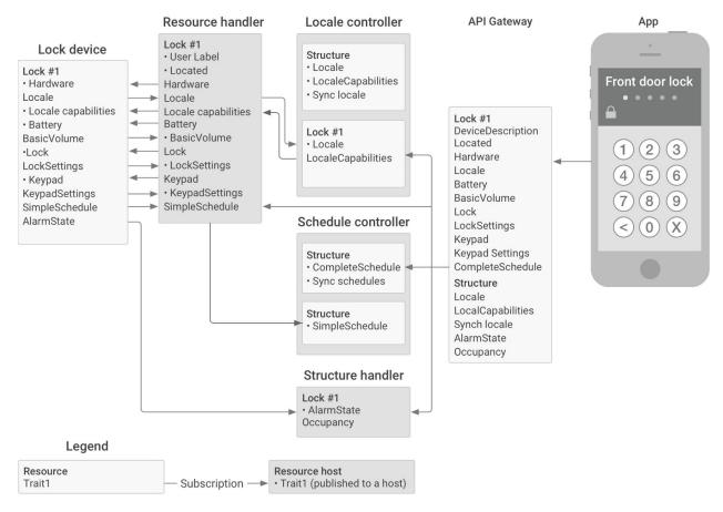
The distribution of traits between a device and various controllers is maintained on the resource definition using options that describe the configuration. The configuration defines which traits of the resource are code-generated for the device, and which controllers must be invoked to complete the implementation of the resource.
