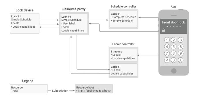
In the diagram, the App is communicating with different hosts to access the various traits of the lock and structure resource. The Nest Service collects all of these traits into a single unified resource view, and presents the resource view to clients. The app doesn't need to understand the distributed system servicing each resource, but it can talk to a single API exposing all the resources to which it has access.
